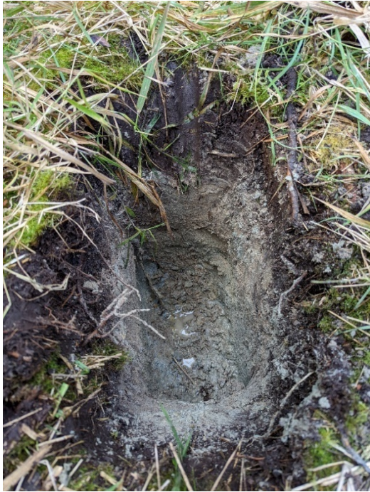
Photo B17 View of test pit excavated by hand shovel immediately west of berm.
