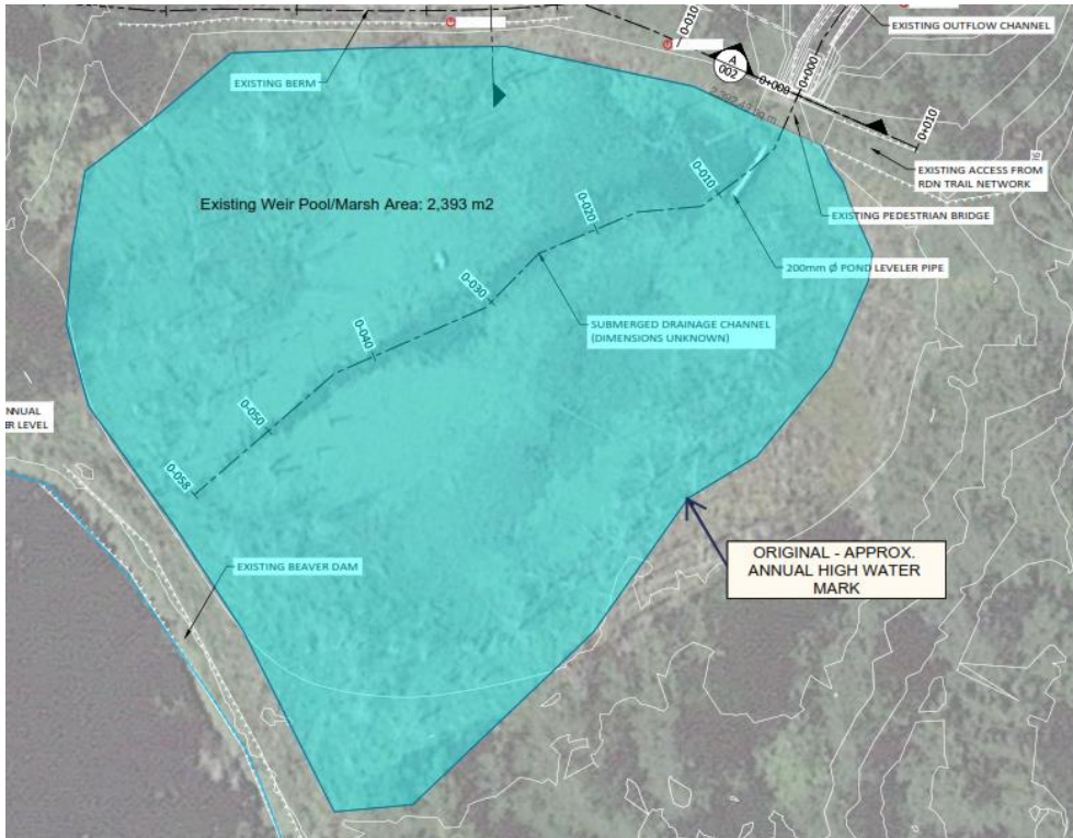
Figure 3-2. Proposed weir pool/marsh area (to new estimated annual high-water mark) after dam decommissioning
