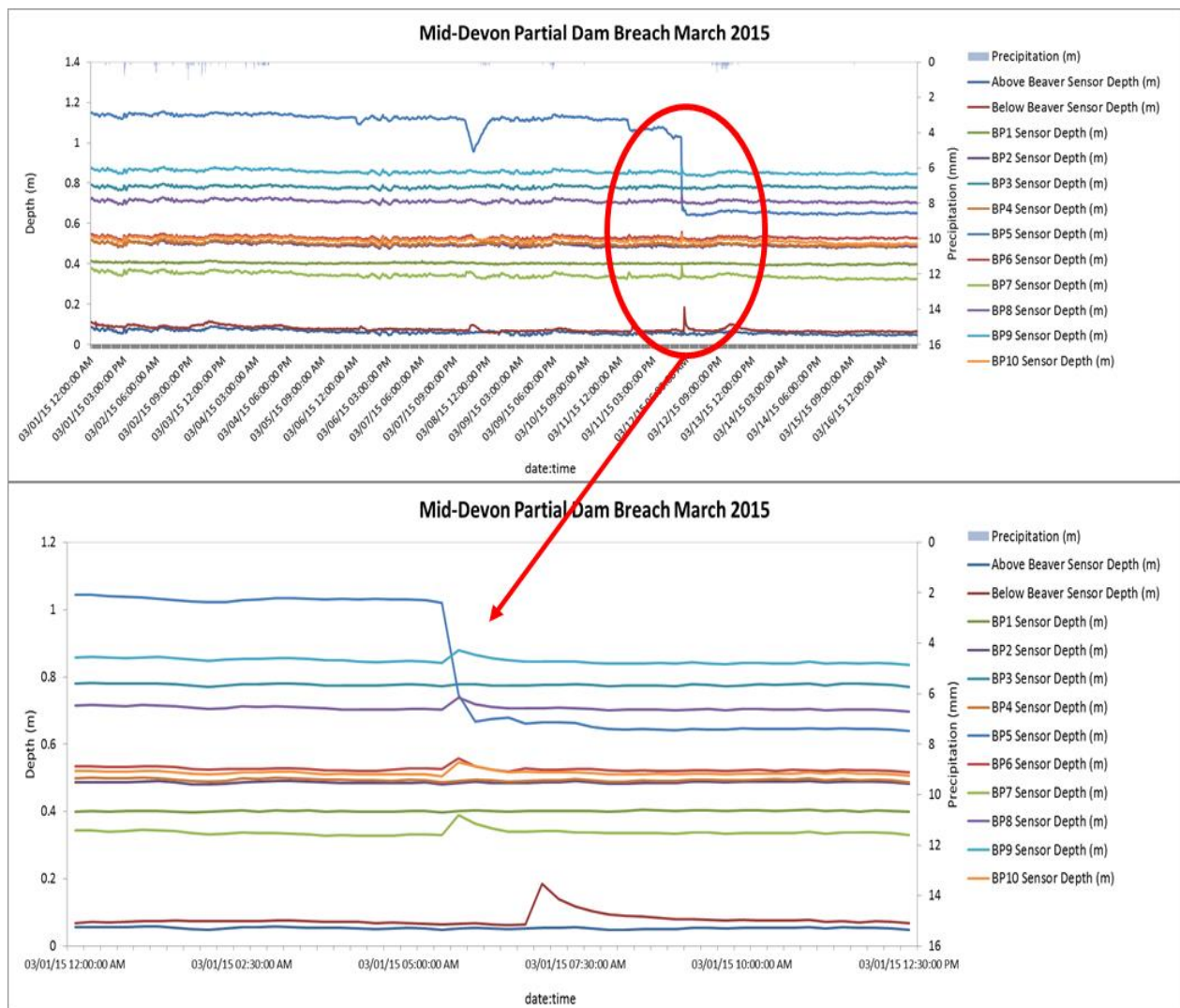
Figure 7. Downstream impact of beaver pond breach in a mid-sequence pond (BP =beaver pond). Blue line showing large drop on 12 th march is Pond 5 in a sequence of 10 ponds. Effect can be seen to propagate through/be dissipated by beaver ponds 6 -10 resulting in a minor and temporary increase in downstream water level (Below Beaver sensor – red line).
