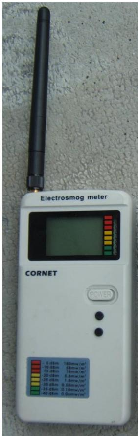
1. CORNET ED-85EX for electromagnetic field power density. Manual ED-85EX2 V.3.1L.
