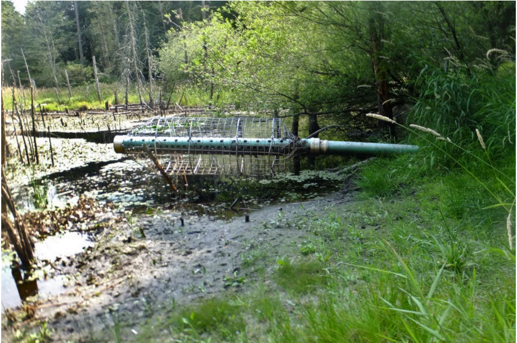
The Clemson leveller is a good design. The beaver has shown limited interest in attempting to block it. Its capacity is just too low for this application.
