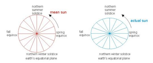
The figure on the left (red) shows the movement during the year of the fictitious mean sun. At the centre is the earth. The plane of the mean sun's orbit is the same as the equatorial plane of the earth (there are no seasons), and the sun moves around the celestial equator counterclockwise in a perfect circle and at a constant speed.
