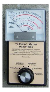
The meter has three orthogonal axes for electric and magnetic fields, which eliminates sensitivity to field polarization.
