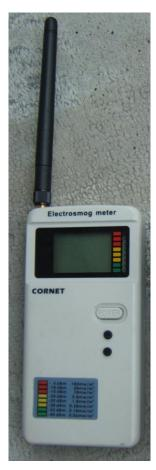
1. <u>CORNET ED-85EX</u> for electromagnetic field power density. Manual ED-85EX2 V.3.1L.
